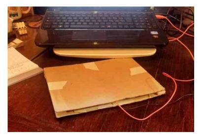
stack the cardboards with aluminium foils face to face, and attach with tape
